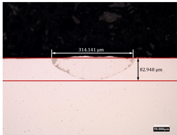
(a) Measurements of melt pool width and depth.
