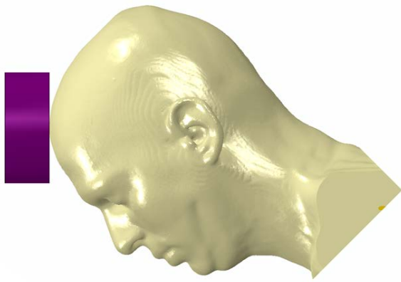
Figure 3: Experimental setup of Nahum et al. , a) Representative impactor shown impacting NRL-HFHM at a 45 degree incline, b) Normalized impactor force over time.
