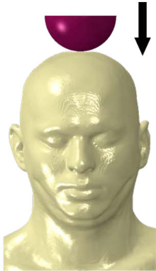
Figure 14: Schematic of case 7 in Yoganandan et al. experiment showing a) impact geometry with the hemispherical anvil and the direction of impact, b) Side view of the skull with red spot denoting the fixed region around the internal auditory meatus on both sides of the skull.
